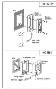
After fix the rear bracket with 4 screw, put the Door Camera into the grooves of rear bracket, and then fix it with hexagon screws and stick the finishing materials.
